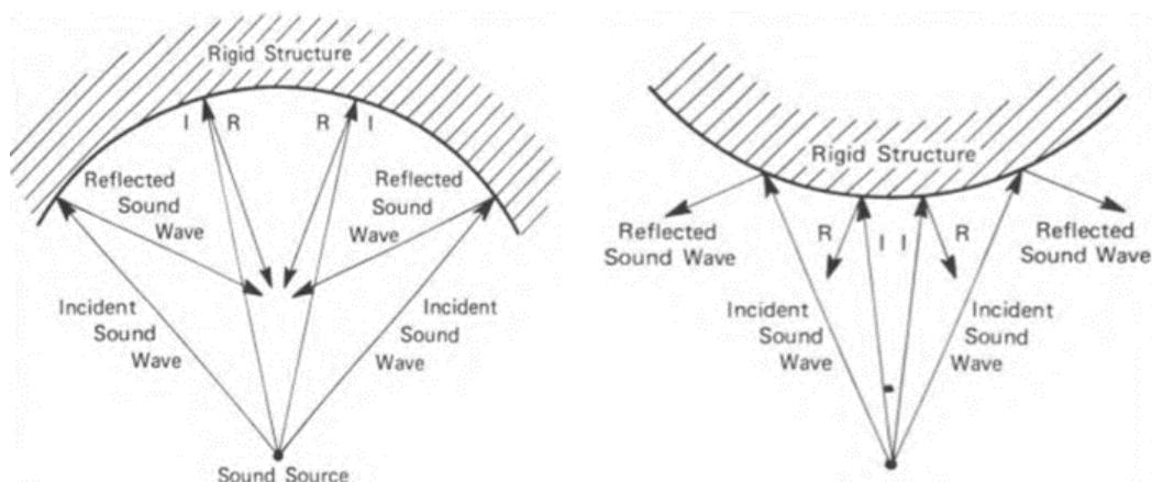
Figure 1. Reflections of sound rays on the curved surface; a) concave b) convex (Ginn, 1978)
