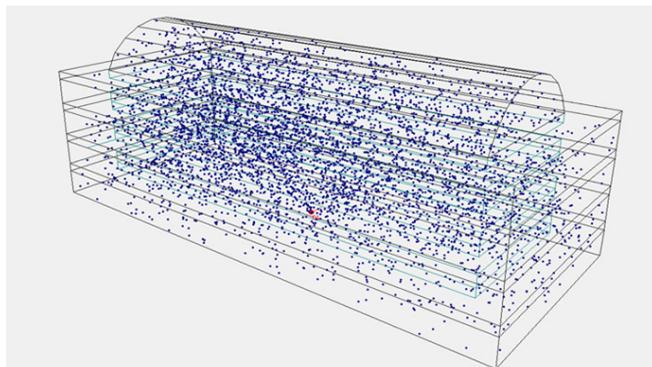
Figure 2. Example of the validation process using water tightness test by 3D billiard in the model room of F3 rectangular atrium with barrel vault-shaped skylight
